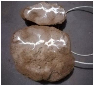
图 2 化学注浆固砂体整体形态特征 Fig.2 Morphological characteristics of chemically grouted sand
