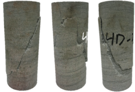
(c) 空心圆柱灰砂岩单轴压缩破坏形态
