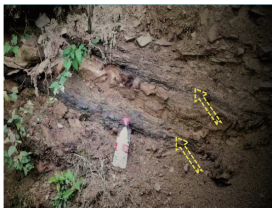
图 11 贵州张家湾普洒滑坡原始坡体坡脚处出露的煤线 Fig.11 Outcrop of the coal seam at the slope toe the original Pusa slope in Zhangjiawan Town, Guizhou Province
