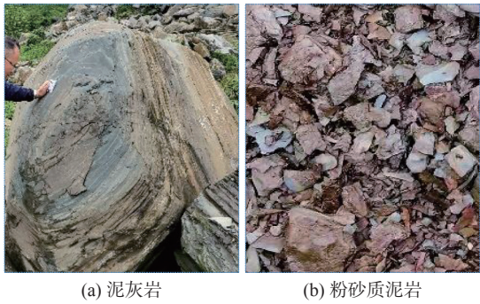
图 6 贵州张家湾普洒原始坡体中泥灰岩与粉砂质泥岩的物理风化 Fig.6 Physical weathering of the marl and the silty mudstone in the original Pusa slope in Zhangjiawan Town, Guizhou Province
