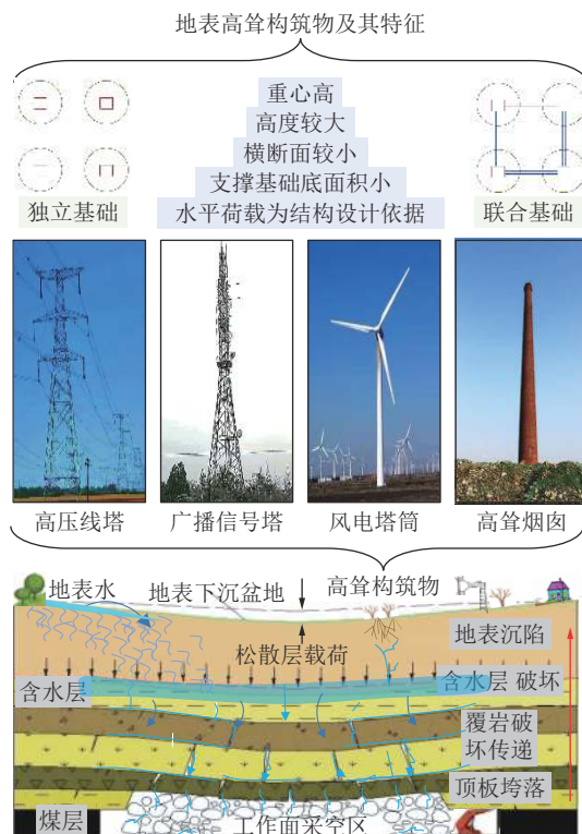
图 1 煤矿长壁开采引起地表高耸构筑物损坏示意 Fig.1 High-rise structures damage due to longwall mining
