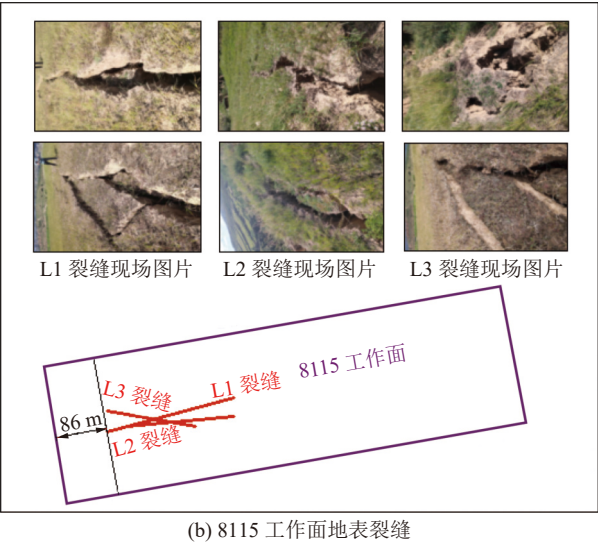
图 17 工作面地表变形状态 Fig.17 Surface deformation state of coal face
