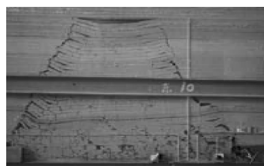
图 9 砌体梁结构失稳 Fig. 9 Structural instability of masonry beams
