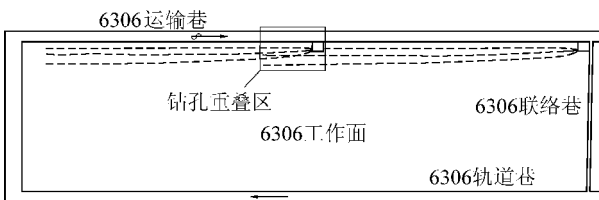
图3 6306工作面高位定向钻孔成孔轨迹示意 Fig.3 Trajectory diagram of high position directional drilling hole in No.6306 working face
